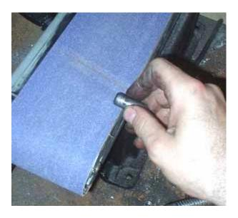
The pin was binding. Experience has taught me that any hangs up or deviations will result in too much force and the bracket will break at the tack weld and I have to grind everything clean again. I sand off the burr on the pin. The belt is not even running, I'm just rubbing it against the stopped belt.
