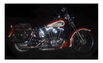
Here's the show side of the bike. I threw the sprocket cover in the trash and fabbed up a steel bracket for the kick starter. I mount the battery in the front in that swoopy bracket you can just make out. I need to redesign it though-- this fender just touches it at full jounce. That's a project for another day.
