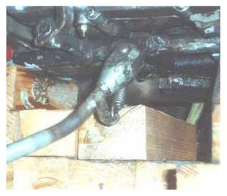
A pathetic simulation showing how I bent the side side stand with a torch to make up for welding the bracket on at the wrong angle. My dad used to joke about golfers who had a bad slice "fixing" their slice by just standing at an angle to the fairway. They still sliced, only the ball went down the fairway kinda sorta. Same stupidity here. I should have ground of the bracket and started over. Actually the real cool way to fix this is to pull the motor and ........
