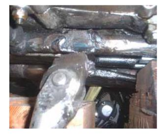
Here's a shot down under the primary cover where the side stand mounted. You can see the lousy weld.
