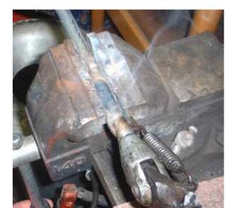
While it's still red hot and spewing deadly cadmium fumes I clamp it hard in the vise twice at 90 degree rotations to straighten it that last little bit.
