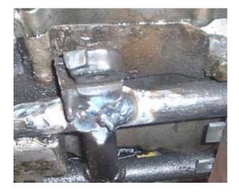
Here's the second tack weld. It's a little droopy but some of that glop is flux that will break off. I did a little one with the clamp setup and using my left hand I could get the stick in for a little tack. I then took the pin out (easily due to all that deburring) and did a pretty big tack.
