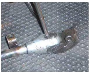
I won't show the whole fiasco where I tried to epoxy the bracket to the frame in the right position so I could then weld it. It didn't work so I peeled off the epoxy and tried to fixture the thing up. I took out this screw so I can take the stand apart easily once I tack weld the bracket.
