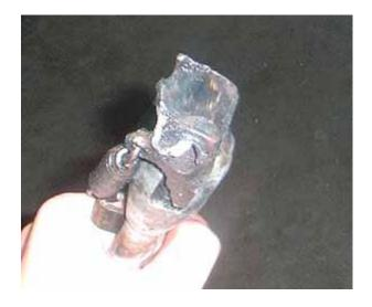
Here's a view of the first level clean up. Still a lot of work to do. There is a little undercut by the spring that I tried to bridge before, but know I decide to grind the undercut way deep so I can get a stick in there to weld the actual pad.
