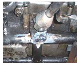
I put the stand back on to eyeball it and see how it looks in the up and in the down position. I compare the gap from the top of the pin to the engine case to another bike.
