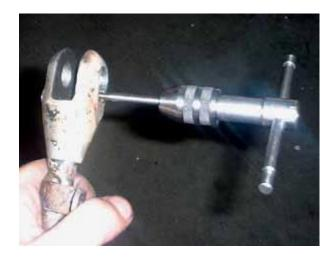
Always misery and suffering with Harleys. I guess it builds character. The little stop screw that holds the pin in won't thread in easily. I clean up the threads (12-24) and run the screw into a die.
