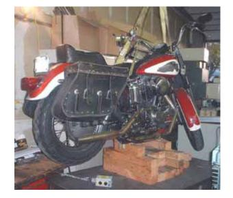
Do you wonder how I get the bike up on the old desks I use to work on? A hoist on the roof beam. The desks legs are dropped into big steel tubes I welded casters to. I wheel the desk under the hoist, lift the bike and .....
