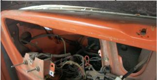
The 1979 truck brought metal up under the plastic to get those free grounds. Once I pointed out we needed to add wires, that pretty much made the cost basis a wash. Wire cost back then was a penny a foot and a penny for each connector pin on the ends. That was design cost, and a penny got management really worried. The cigarette lighter needed even more expensive heavy-gauge wire. I was not popular with management, but it was not my mistake.
