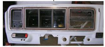
The 1979 Ford truck instrument panel had a plastic instrument cluster in a steel panel.
