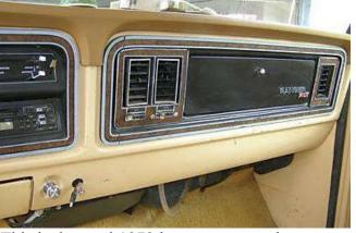
This is the steel 1979 instrument panel we replaced with the 1980 plastic panel.
