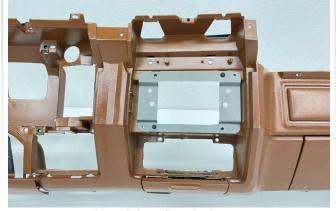
One we got the wiring fixed, the test group noted the plastic panel flopped all over the place. We had a test engineer, Phil "Crash" Krushka. He took pride in running the truck over the Belgian Block shake test. He once lost a tooth filling he beat on the truck so hard. So now Body Engineering had to add steel braces and stiffeners everywhere. Now the cost savings had gone from a wash to a cost penalty.
