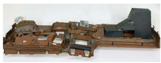
You can see the insane complexity of the injection-molding tool needed to mold the panel. This meant that once the tool was cut, there was no chance they could make any major changes, and remember, this whole fiasco was supposed to be a cost savings.
