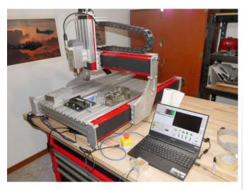
I paid around \$9000 for an Avid Benchtop Pro mill, in the 2 foot by 3 foot size. It was a lot because I got the Avid high-speed spindle package, and the NEMA-34 motor upgrade. I also ordered their tool probe that helps you set the tool height and find "part zero" on the workpiece when you set things up.
