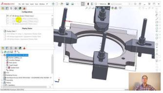
The right way to do fixtures is in an assembly. The screenshot above shows that same part now in an assembly, with four clamps added. Note that I also modeled the hold-down bolts, since you are even more likely to break a tool on those, though you might get lucky and just break the bolt before ruining your spindle.
