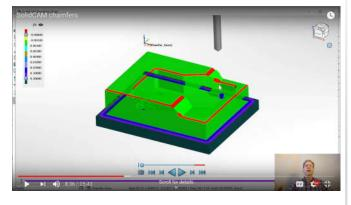
Above you see the simulation of the automatic chamfer recognition operation. Note that it has decided to do both the outside of the part and the inside of the pocket. Also note it can only do the flat chamfers, it can't handle the slopes. All the chamfers appear as red gouges since the chamfers were not in the part model, this is using CAM to add chamfers.
