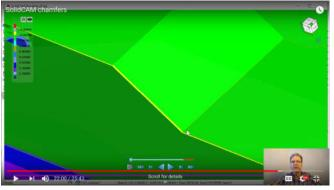
You can do a 3D chamfer as a subset of the "Contour 3D" operation. Because of the geometry of a slanted edge meeting a cone, the chamfer will be a bit wider on the slopes. This is minimized if you do a small chamfer (0.005") with the cutting diameter of 0.005", right at the tip of the tool.
