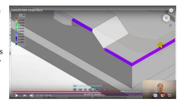
Using a manual "Profile" operation to do the chamfer lets you pull the geometry back from the slopes to prevent the gouges. I see that the chamfer on top is ending a bit soon, so I also should have extended the geometry on that edge. You could also use lead-in and lead-out to to do this, but then you could not do both chamfers in one operation. Here I did no lead-in or lead-out to eliminate the gouges on the slopes.
