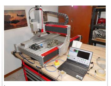
With the top operations all fixed up, I went to do the bottom of the part. I am pretty sure I got part-zero defined right, set to the bottom corner of the part. This would have to mean finding the Z height of the parallels that the part is sitting on. I assume I could have a part-stop setup so that I would not have to find X- or Y-zero again, I could use the previous ones.
