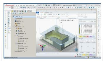
Here I left the "System compensation" of the roughing pass set to "right" and it bombed the endmill through the part. It did a similar carveup when I tried a simple 3D slope.
