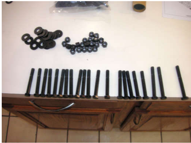
The 3/8" bolts also come in slight length differences.
