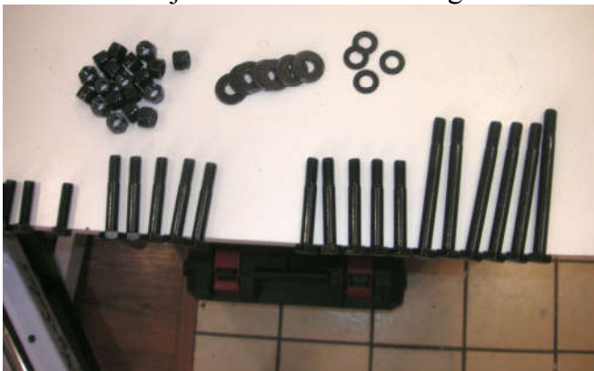
Be sure to lay out the bolts so you can see all the different lengths. These are 1/2-inch bolts.
