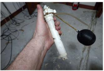
The toilet valve that broke, blew the cover off the tank, and started to flood the room.
