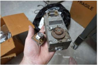
A defective gas valve from the heater in my shop circa 1995. It was a loose rivet. I wanted to do a write-up about little things breaking systems. Maybe another day. Now, it just felt so good to add it to the trash bag.
