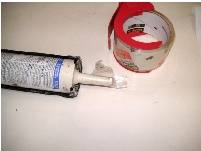
You can seal the caulk with clear tape.
