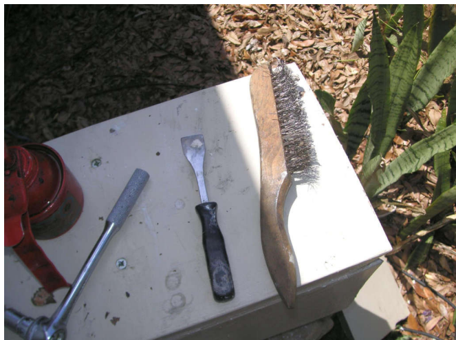
It got really messy, so I used a gasket scraper and a wire brush to clean off the excess silicone. Next time I will be more careful.
