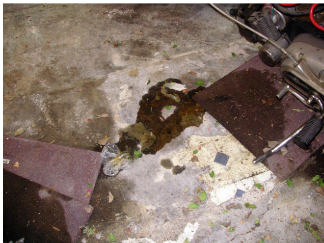
The day after "fixing" the oil pump, this giant oil spill is on the garage floor.
