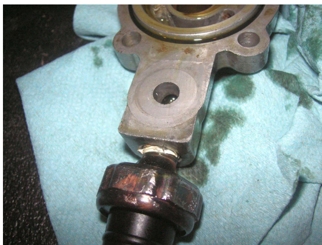
This is where the missing O-ring seals against. I make sure it is clean and flat.
