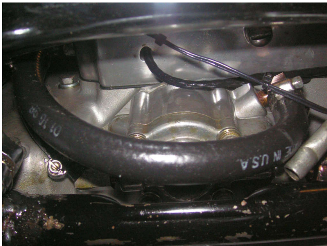
You can see a stain on the cover from where the oil was leaking past the missing O-ring.
