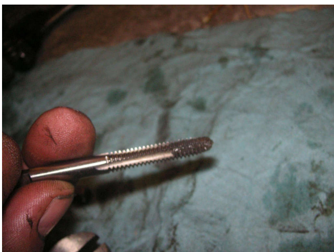
The tap came out filthy. I chased the other three threads right after seeing this.
