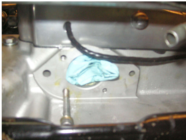
I blocked the drive hole with a paper towel so no dirt would get in the gearcase.
