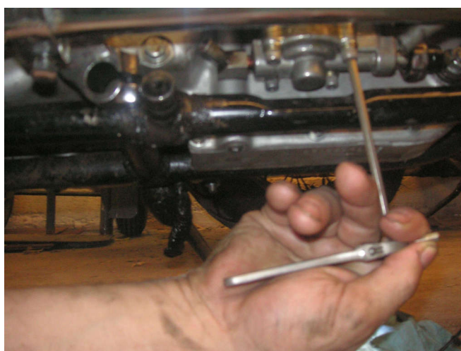
Laying on the garage floor, I installed the oil pump with that Crescent wrench & Allen key.
