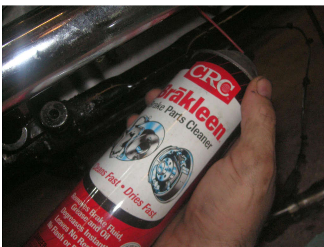
Brakleen gets any oil or grease out of the tapped holes for the oil pump.
