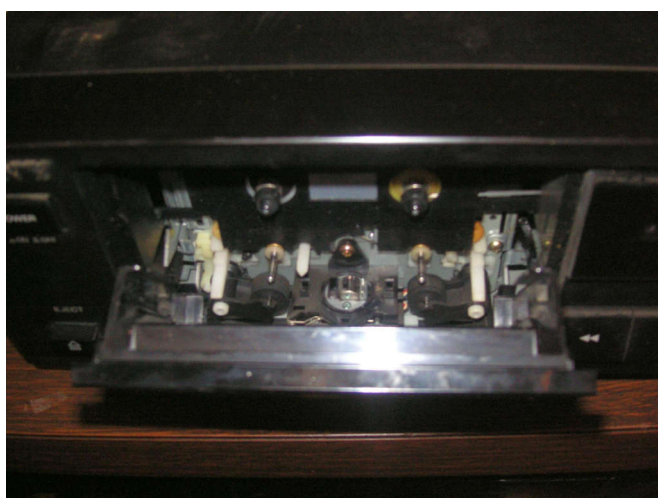
I learned to keep cleaning the heads and capstan with isopropyl alcohol.
