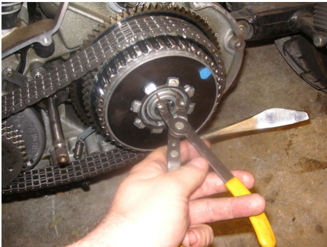
I wear safety glasses any time I install C-clips. This one holds in the clutch adjuster. Those old Craftsman snap-ring pliers worked for 40 years.
