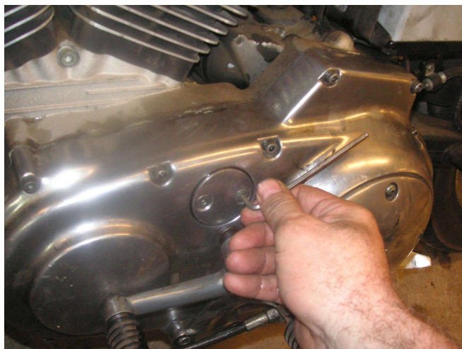
With the O-ring in, button up the access cover to the primary.
