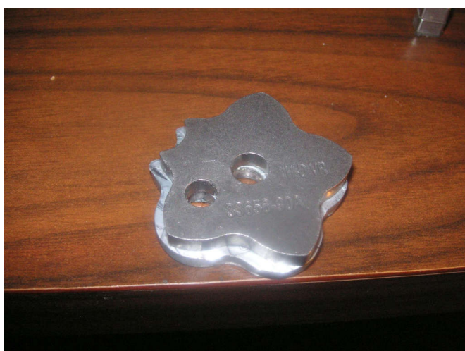
The new plate is smaller, thinner, harder and heavier than the old detent plate.
