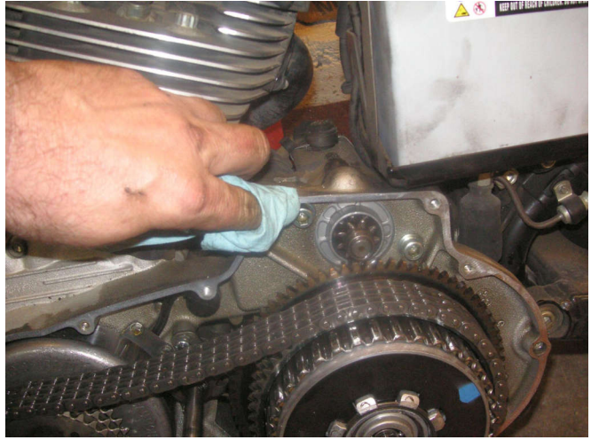
I clean the gasket area. Feeling it all around is important to make sure it is clean.
