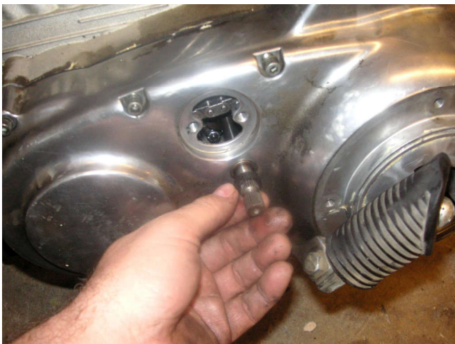
A rubber sleeve goes over the shifter shaft. Not sure why, it's not a seal.
