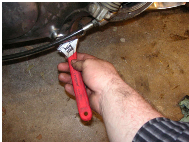
Feeling the chain inside the access cover, you can adjust the stud, then tighten the jam nut.
