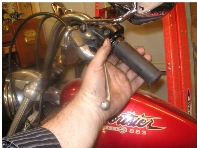
You get a feel for how the clutch should work. I have adjusted for cable length with that cable bushing, back off the screw until it feels OK.
