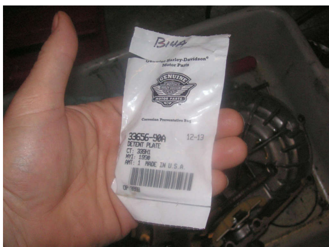
Here is the new detent plate. Part# 33656-90A. The "A" means it was an upgrade.
