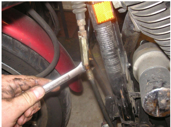
This is where you adjust the clutch after you run the clutch screw all the way in.
