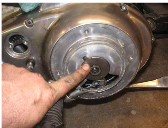
The adjuster does not sit right with the cable hook installed that way.
