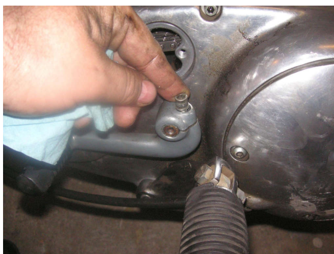
The bolt then goes in and gets tightened. The bolt has to be out to get the lever on the shaft.
