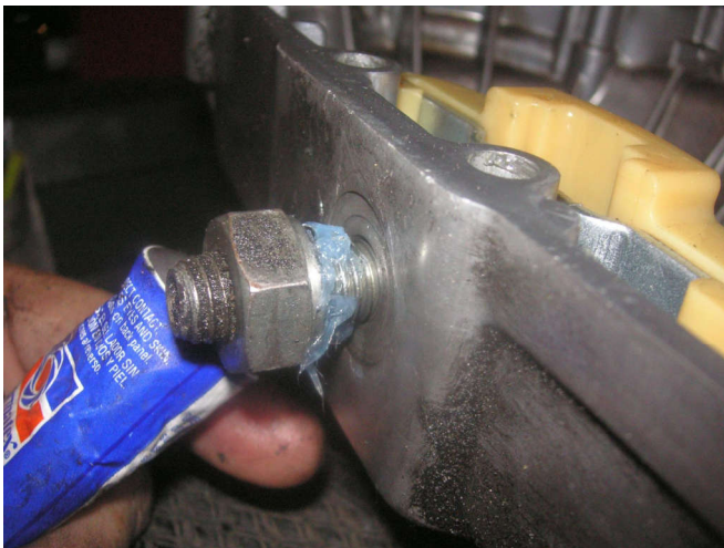
A little blue RTV gasket silicone around the stud keeps a leak from forming.
