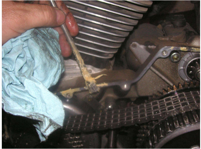
I put lithium grease on the gasket surface to hold the gasket in place..
