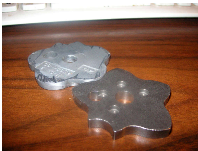
The new plate is thinner. You can see the scars on the old plate from rubbing the clutch basket.
