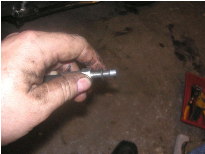
The detent plate kit comes with a new O-ring for the clutch cable. Lay on your belly to make sure the cable is not cross-threaded in the cover.
