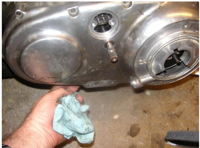
You have to reach up and push the chain up over the adjuster to get the cover installed.
