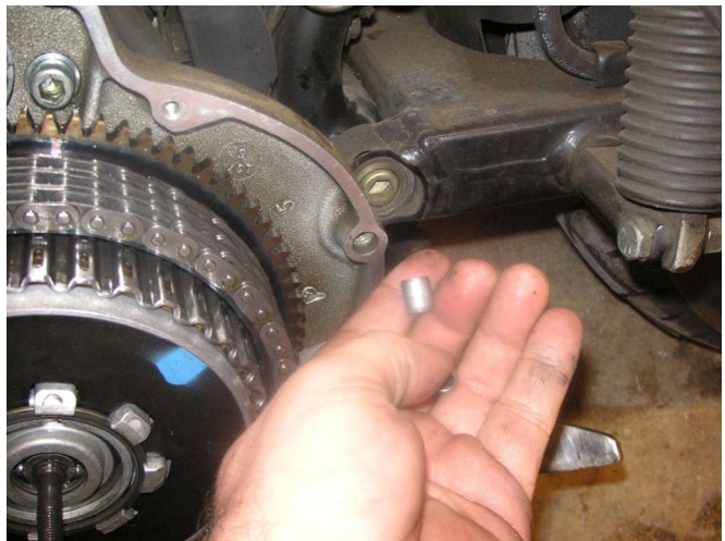
Don't forget the locating dowel in the back of the primary.
