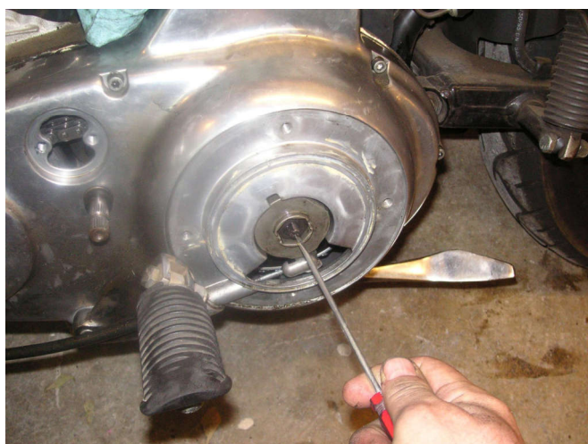
A screwdriver adjusts the center stud. You can fiddle with this after you ride the bike.
