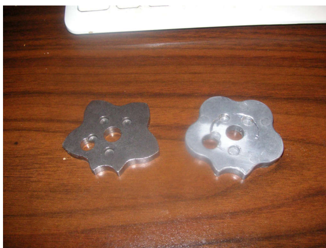
The new plate looks like it tries to keep the bike in gear, the dips are deeper.
