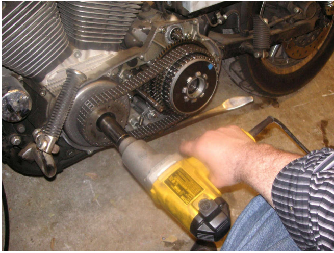
The sprocket nut is 1 1/8 inch. I used a touch of blue Loctite here as well.
