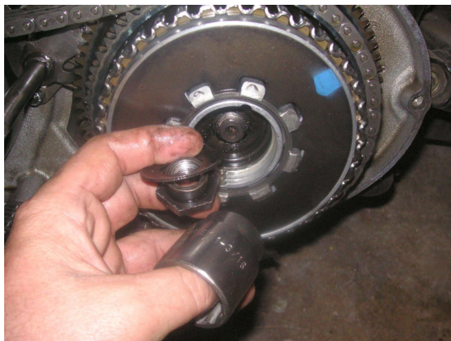
The clutch basket nut is 1-3/16. Don't forget the flat washer.
