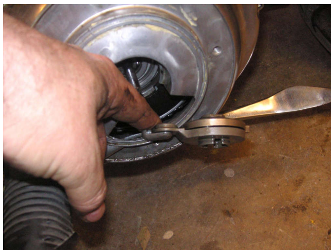
Flip the cable hook like this when you install the clutch ball ramp assembly. Now it will line up correctly.
