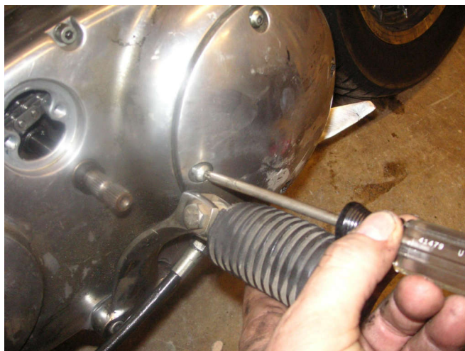
You can button up the derby cover, making sure the O-ring is positioned, I use lithium grease.
