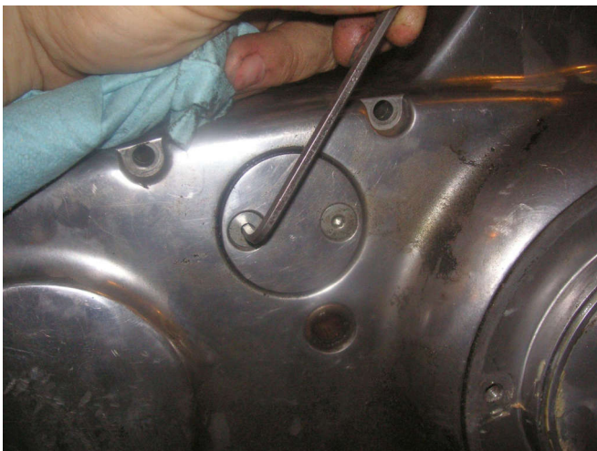
Back out the access cover so you can adjust the chain and add oil.
