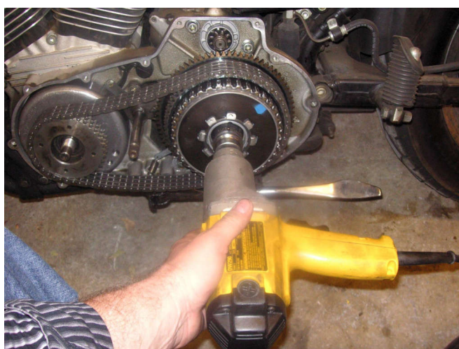
My corded DeWalt 1.2-inch impact runs the nut on. I don't rap in on too hard, the Loctite works.
