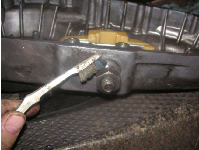
I clean around the chain adjuster, and make sure it is backed all the way out.
