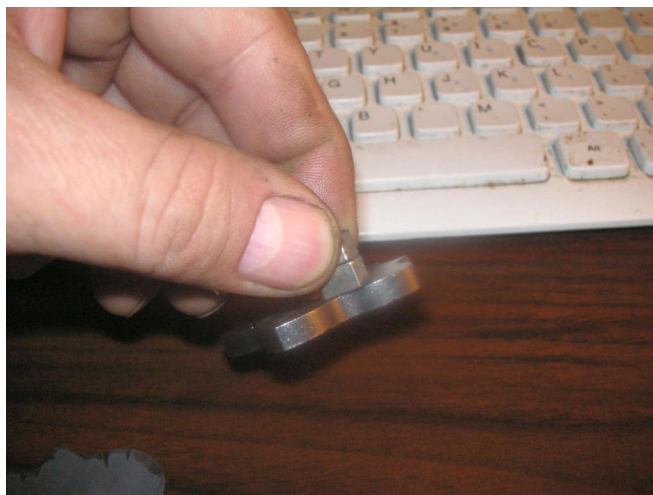
The new one is powdered steel, a magnet attracts is. The old one was zinc or pot metal.
